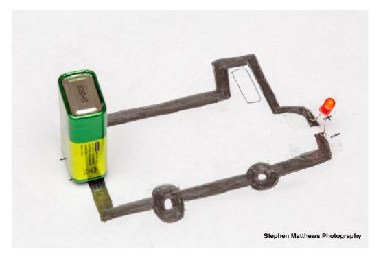
Try experimenting with drawing lines of different lengths and thickness. Graphite is quite low in conductivity, so if your lines are too long, the LED will be dimmer. Experiment to see what kind of line gives you the best results.
