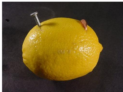
By inserting the copper coin and the nail into the lemon and connecting wire to the nail and the coin, the lemon can be used to replace the battery in a simple circuit. You can add more rows of coins and nails in the same lemon.
