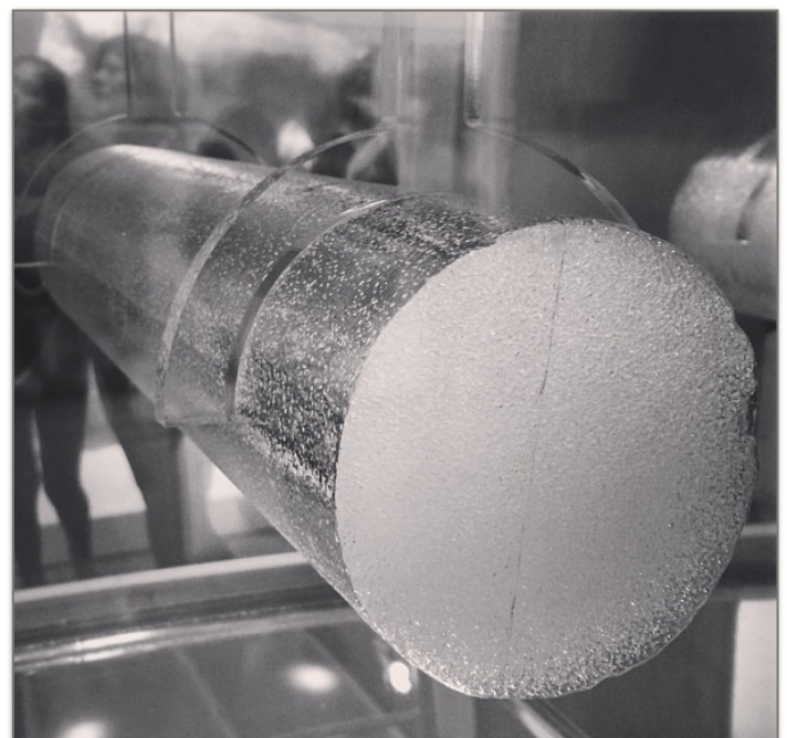
Above: An Arctic ice core sample. Air bubbles can clearly be seen in the ice. Photo by Stefan Leijon
