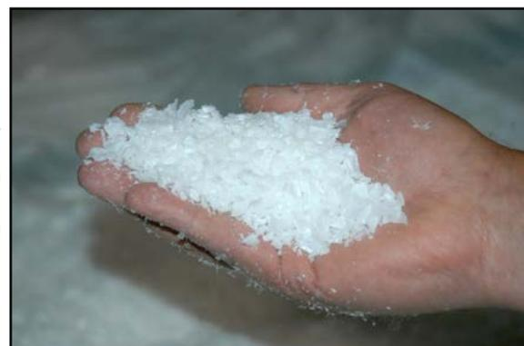
**Above:** Recycled plastic is broken down into flakes before being melted and moulded into a new shape. Photo by Wisconsin Department of Natural Resources.
