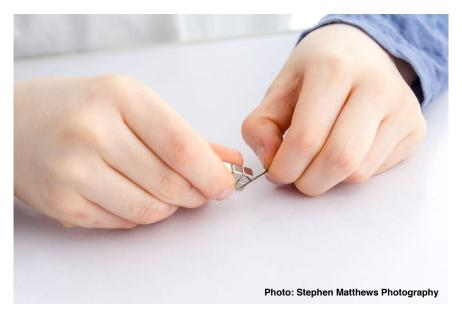
You can use a magnet to do this, but, if you don't have one, you can rub the needle against an iron nail or even your own hair! By doing this, you are actually aligning the atoms of the needle. An explanation of magnetism can be found here (You tube clip, supervision recommended): <a href="https://www.youtube.com/watch?">https://www.youtube.com/watch?</a> v=s236Q1nuWXq
