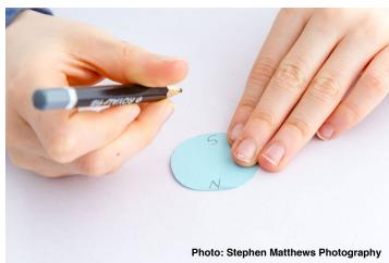
Next, draw and cut out a shape to be your compass. Label it North and South. To magnetise your needle, you'll need to stroke it many times in the same direction against your magnetiser. Using the north pole of the magnet and stroking this towards the point of the needle will cause the needle point to face North.
